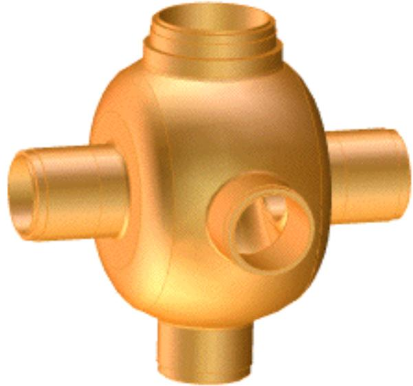
Figure 1. CAD model of 1.5 GHz cavity
