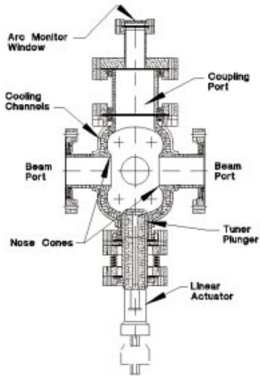
Fig. 4. Cross section of the 1.5 GHz harmonic cavity.
