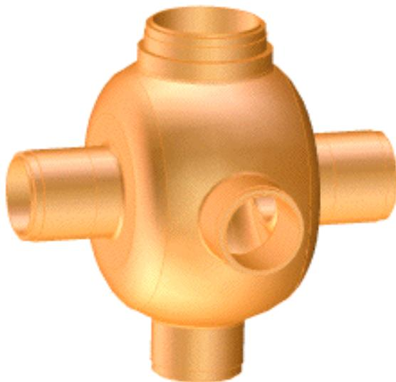
Fig. 5. Three dimensional model of the harmonic cavity.
